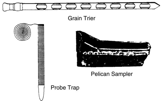
**Figure 9. Standard Sampling Equipment and WBII Probe Traps.**
